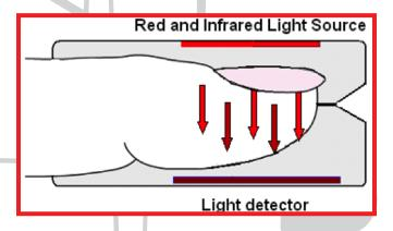
it reaches the light detector. Oxygenated haemoglobin (oxyhaemoglobin or O2Hb) absorbs more infrared light than red light. Deoxygenated haemoglobin (Hb) absorbs more red light than infrared light. By comparing the amounts of red and infrared light received at the light detector, the pulse oximeter calculates the oxygen saturation and displays it on a screen as a percentage.
